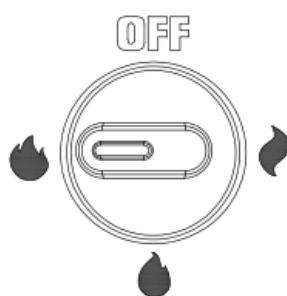
4. Turn the switch to "OFF", the heater is in off mode.
