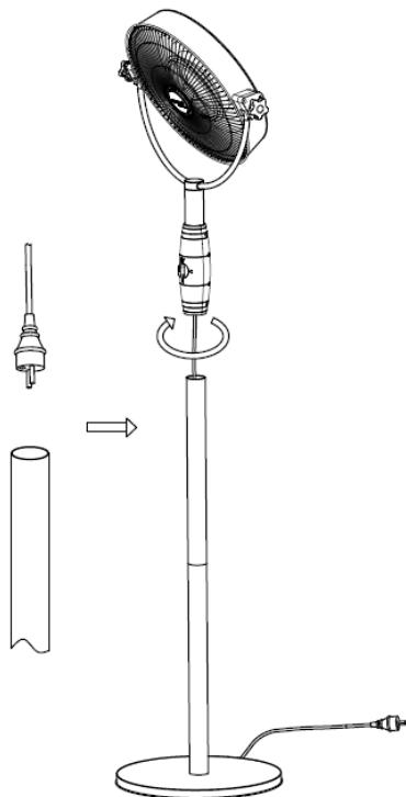
Step 4: Carefully pull the power cord out of the base as far as possible. Secure the power cord under the base with the 4 M4 nuts provided.
