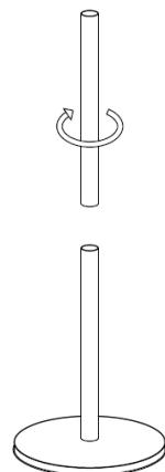
Step 3: Insert the power cord plug through the middle pole, the bottom pole and the base and connect the heating head by screwing them together.
