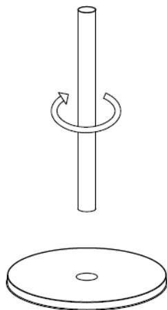
Step 2: Connect the middle pole to the bottom pole by screwing them together.
