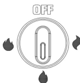
3. Turn the switch to “🔥”, it means the heater is working and on the maximum heating position (2100W).
