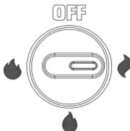
2. Turn the switch to “🔥”, it means the heater is working and on the medium heating position (1200W).
